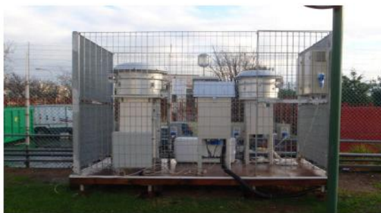
Air sampling station set up at NSA Naples during the air sampling period. This is one of nine stations constructed by the Navy for the Naples Public Health Evaluation.
